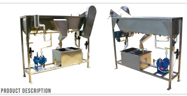
The Alcohol Float is a specially designed machine that will remove pecan weevil larva from nutmeat. Although operating this float requires a liquor license, commercial processors that own these machines believe that is well worth the trouble. The float fluid is a mixture of ethanol and water. This mixture has a specific gravity such that allows the nutmeat to sink, but the weevil larva floats. The larva is skimmed off of the surface of the water, and the nutmeat is conveyed away with a belt.
